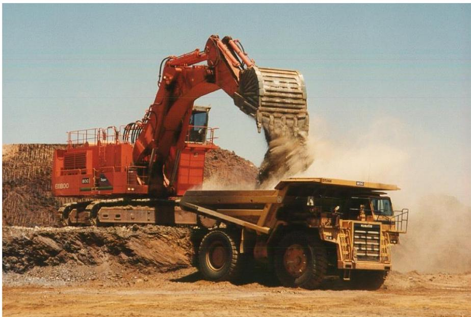
*Figure 6; loading ore at Wodgina mine, Australia.*
