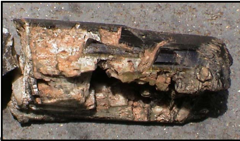
Figure 2) Tourmaline crystal from Malkhan, Russia. The central portion of the crystal has been altered and replaced by K-feldspar. The exterior rind appears pristine. The specimen is 4 x 7 cm.
