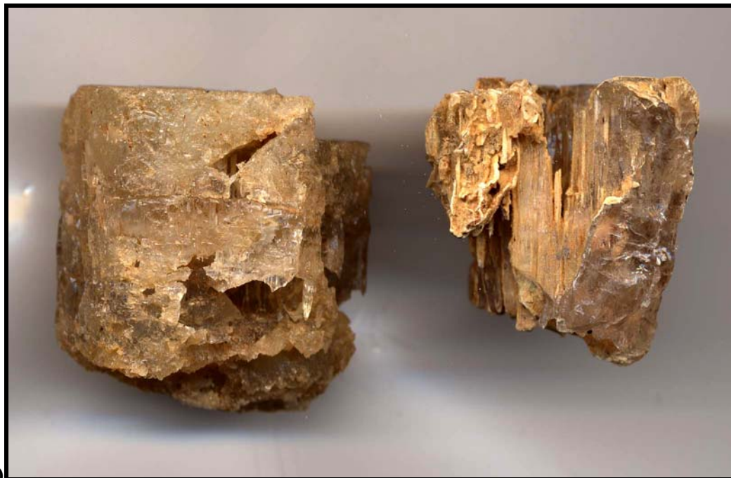
Figure 19) Cavernous goshenite beryls from the Garnet Ledge, Little 3 Mine. Both crystals show extensive dissolution features on the interior and exterior. It is possible that both beryl and intergrown quartz have been removed.
