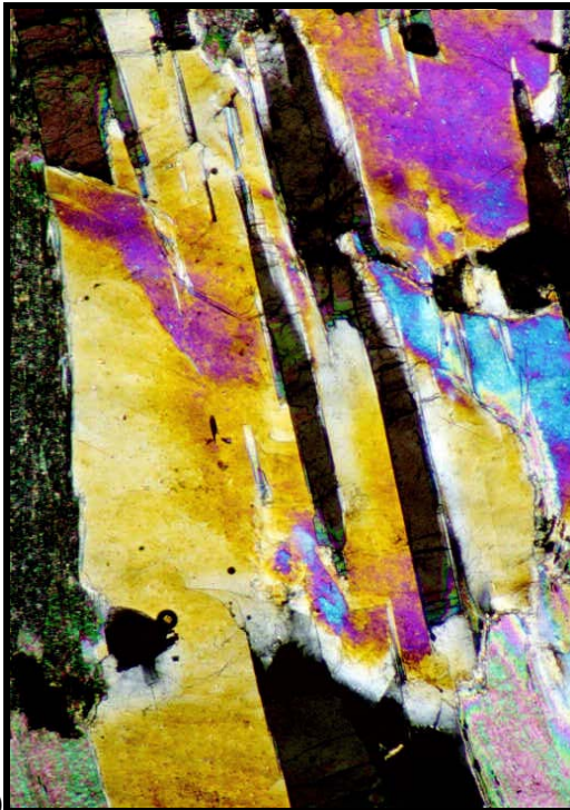
Figures 13 and 14) Photomicrographs of a thin section of a copper bearing elbaite altered to lepidolite from the specimen in Figure 12. The crystal is cut parallel to the C-axis. Mineral identification by XRD at the University of Calgary.
