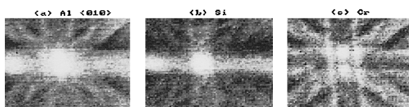
FIGURE 6. Experimental [010] ICP showing (a) Al (1441,705 and 90,15), (b) Si (606,235 and 90,15), and (c) Cr (433,152 and 80,10).
