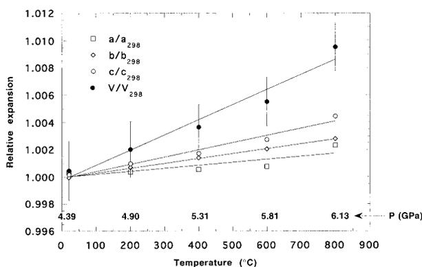
**FIGURE 4.** Thermal expansivity of zoisite at constant load (3500 kN). Error bars are 95% confidence limits on  $V/V_{298}$ . Equivalent error bars on the individual cell parameters would be approximately one-half the size of those on  $V/V_{298}$ . Pressures at each temperature are shown.
