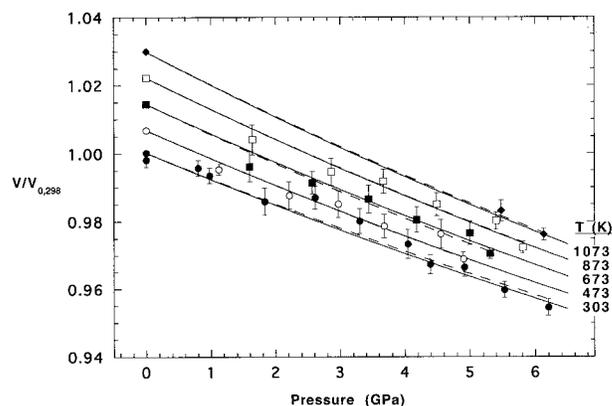
**FIGURE 5.** Zoisite volume data used to determine bulk modulus as a function of temperature. Error bars are 95% confidence limits on  $V/V_{0,298}$ . Points with no error bars are calculated from Equation 2. Dashed curves are Murnaghan fits to the data. Solid curves are model compressibilities (see text for further discussion).
