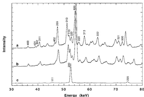
**FIGURE 1.** Energy-dispersive diffraction patterns of zoisite and NaCl in the Walker cell. Detector angle is  $4.84^\circ 2\theta$ . (a). Zoisite at ambient pressure and temperature obtained at the end of the experiment. Zoisite peaks that can be followed through unambiguously to higher pressure and temperature are indexed. (b). Zoisite at 3500 kN (6.13 GPa), 800 °C. (c). NaCl at 1000 kN (0.80 GPa), 20 °C.
