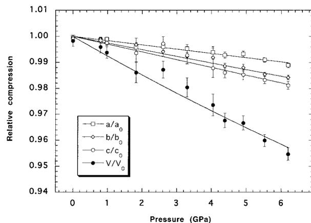
FIGURE 3. Compressibility of zoisite at  $\approx 303$  K. Error bars are 95% confidence limits on the cell refinements. Curve through volume data is the least-squares fit to the Murnaghan equation; the other lines are linear fits to the individual cell parameters. Data points are normalized to 0 GPa values obtained from the fits.
