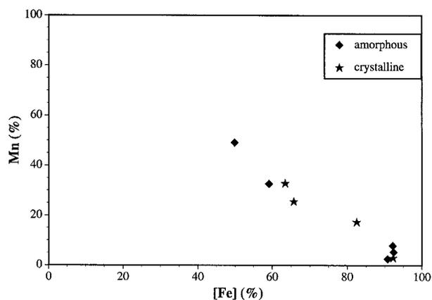
**FIGURE 10.** EDS analyses of amorphous (including coarse filaments) and crystalline material (fine needles) present in dark rock coatings and sea floor deposits revealed the presence of mixed Fe- and Mn-oxides and Fe-oxides containing small amounts of Mn.
