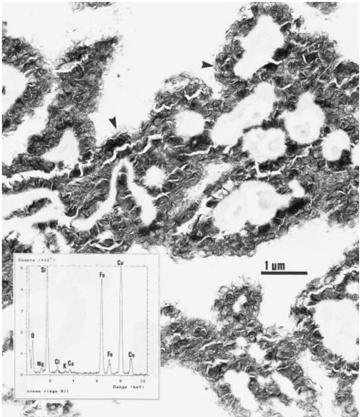
**FIGURE 3.** Unstained thin section of a sea floor deposit showing the presence of fine sheets aggregated around “holes” representing remnants of bacteria. According to EDS analysis, sheets (see arrows) showed an Fe and Si content similar to nontronite (Cu signal is from the Cu-grid).
