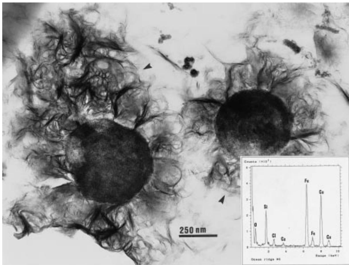
**FIGURE 6.** Thin section of a rock coating showing crumpled sheets (see arrows) growing on spherical nodules, possibly representing completely mineralized bacteria. EDS analyses show an identical chemical composition for the sheets and the amorphous core material, with an Fe and Si content similar to nontronite. (Cu signal is from the Cu-grid).
