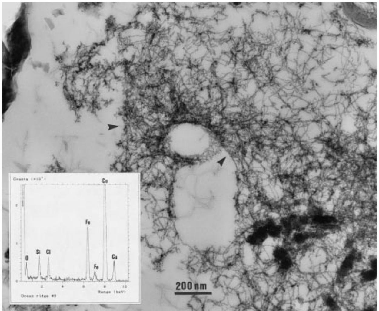
**FIGURE 7.** Bacterial extracellular polymers (see arrows) occurring as fine filaments of Fe-oxides containing small amounts of Si and Cl (see EDS spectrum) in a rock coating. The polymers appear to trap small round nodules also composed of Fe-oxides. (Cu signal is from the Cu-grid).
