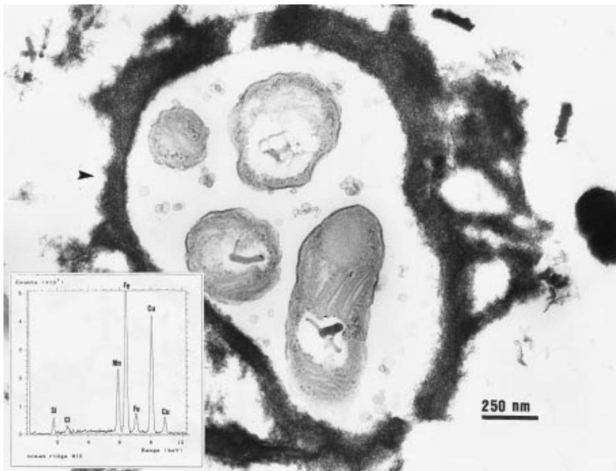
**FIGURE 4.** Microcolony of bacteria surrounded by very fine needles and amorphous material (see arrows) rich in Fe and Mn, with small amounts of Si and Cl (sea floor precipitate) (Cu signal is from the Cu-grid).
