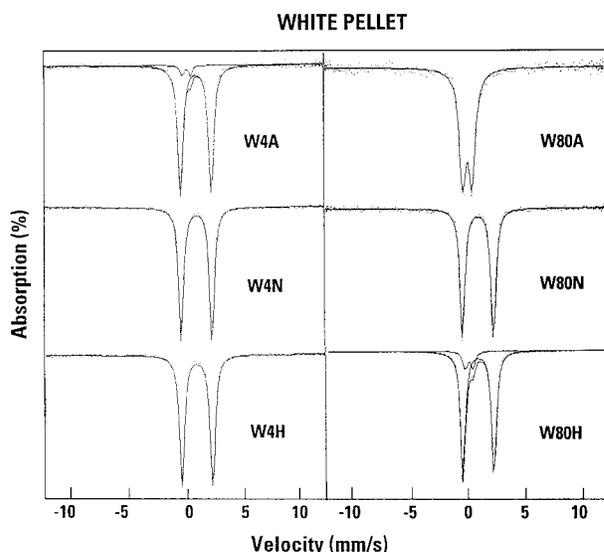
**FIGURE 2.** Mössbauer transmission spectra obtained at room temperature using a white (W) precipitate incubated at 4 °C (4) and 80 °C (80), under air (A), nitrogen/carbon dioxide (N) and hydrogen (H), for 12 weeks.
