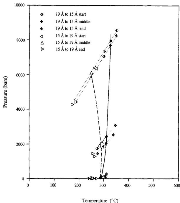
**FIGURE 7.**  $P$ - $T$  diagram of CaSWy-1 summarizes the  $P$ - $T$  conditions for the starting, middle, and ending points of dehydration and rehydration cycles for 19 Å and 15 Å hydrates. The solid line is a visual fit to midpoints of the dehydration process. The dashed line is a visual fit to midpoints of the rehydration process. The distance between the lines indicates the size of rehydration hysteresis. Points collected along the same isochore are connected with dotted lines.
