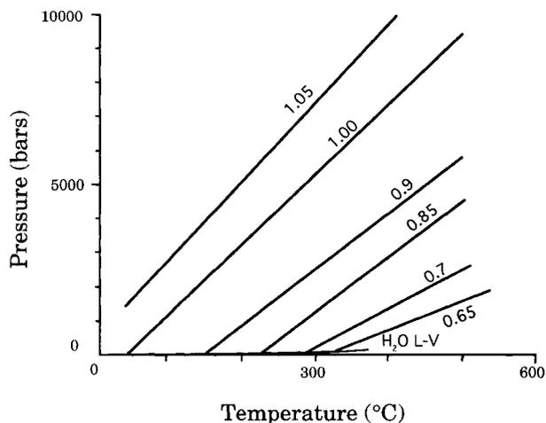
FIGURE 2.  $P$ - $T$  diagram showing the isochores of the heating paths followed during experiments. Numbers next to each line represent the densities of the  $H_2O$  isochores in grams per cubic centimeter.
