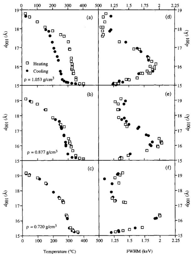
**FIGURE 4.** The  $d_{001}$  values of CaSWy-1 vs. temperature (a–c) and the full-width at half-maximum (FWHM) (d–f) of the 001 peak. The H<sub>2</sub>O isochoric densities are shown.
