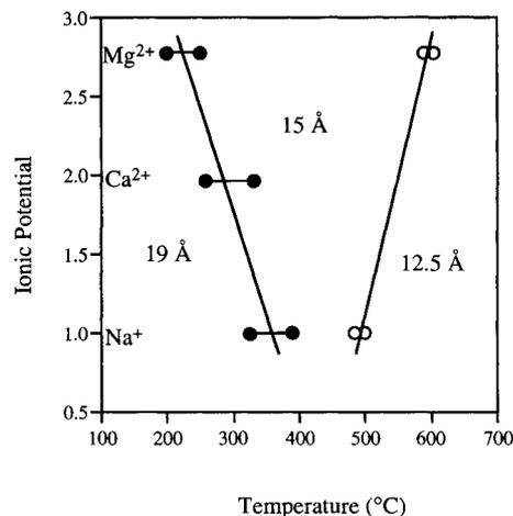
**FIGURE 10.** Ionic potentials (charge/radius) of Na<sup>+</sup>, Ca<sup>2+</sup>, and Mg<sup>2+</sup> cations vs. dehydration temperature for SWy-1 montmorillonite exchanged with those cations. Pairs of connected dots represent the range over which dehydration occurs.
