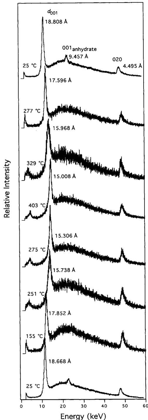
FIGURE 3. Series of energy-dispersive X-ray diffraction patterns of CaSWy-1 during a heating-cooling cycle with isochoric density of  $1.053 \text{ g/cm}^3$ , showing the dehydration process starting at the top and the rehydration process ending at the bottom.
