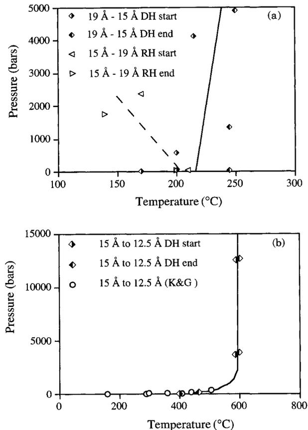
**FIGURE 9.**  $P$ - $T$  diagrams of MgSWy-1 showing (a) dehydration (DH) and rehydration (RH) data between 19 Å and 15 Å hydrates and (b) dehydration data for 15 Å to 12.5 Å hydrates. Our dehydration data are shown as diamonds, and those of Koster van Groos and Guggenheim (1987) are shown as open circles.
