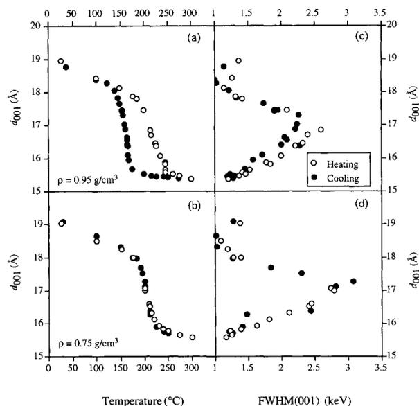
**FIGURE 5.** The  $d_{001}$  values of MgSWy-1 vs. temperature (a and b) and 001 peak width (c and d) for the  $19 \text{ \AA}$  to  $15 \text{ \AA}$  dehydration-rehydration cycles along the  $0.95$  and  $0.75 \text{ g/cm}^3$  isochores.
