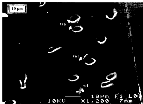
FIGURE 8. The \{11\bar{2}0\} surface (S type), etched for 300 s in 2.5% \text{HNO}_3 (set A). The surface itself is comparatively smooth and crisscrossed by sharp polishing scratches. The track openings (tra) are essentially elongated hexagons, although the precise shape is often influenced by the orientation of the track. Some tracks develop minor additional structures at their intersection with the surface. Near the center of the image, a track at a slight angle to the surface is turning into a residual etch figure (ref). A fully developed residual etch figure (ref) is situated at the bottom of the photograph.
