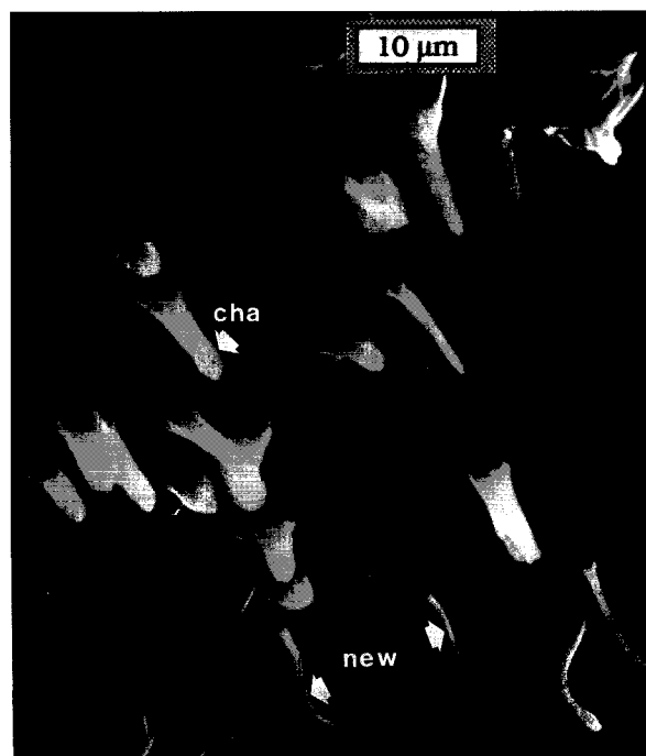
FIGURE 10. Chisel-shaped track channels (cha) in \{11\bar{2}0\} (S type) at intermediate concentration. The more needle-shaped channels correspond to tracks that were added as a result of bulk etching (new). Etching conditions: 300 s in 2.5% \text{HNO}_3 (set A).
