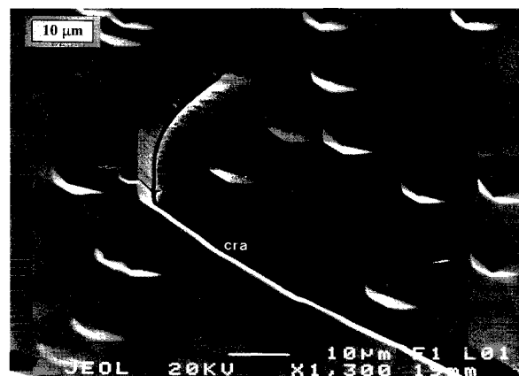
FIGURE 5. A continuous groove with v-shaped cross section along a crack (cra) in a cleaved P-type surface at a slight angle to \{0001\} . Etching conditions: 25 s in 25% \text{HNO}_3 .
