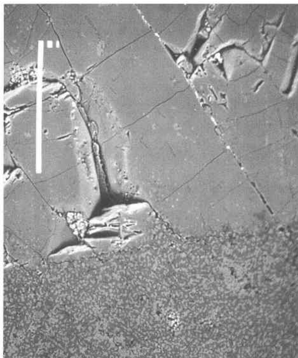
Fig. 2. Backscattered electron image of the experimental product containing the crystals of \text{Na}_{1.8}\text{Ca}_{1.1}\text{Si}_6\text{O}_{14} used for structure determination (Table 1, expt. 2188). The fine-grained material is a mixture of \text{CaSi}_2\text{O}_5 and sodium silicate. The scale bar is 100 \mu\text{m} long.
