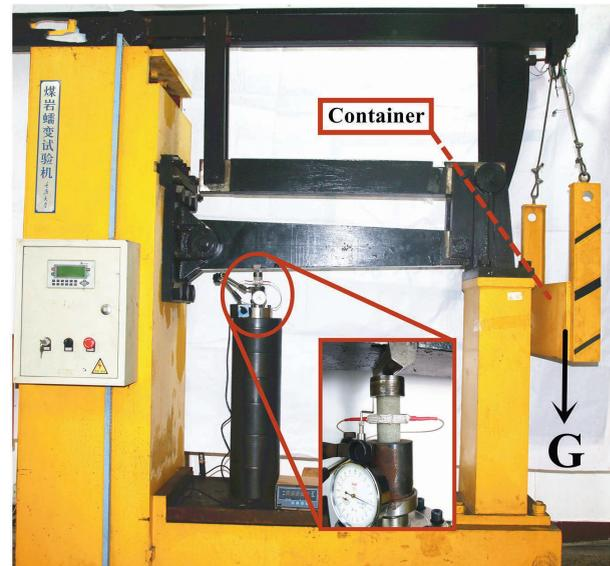
**FIGURE 1.** Photograph representation of the compression arrangement. Oil is poured into the hanging container (on the right) at a constant flow rate; the weight of oil ( $G$ ) is transferred to the lower tilting beam. The samples were placed between the lower tilting beam and a static support.
