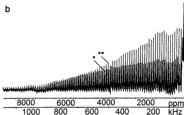
FIGURE 3. (a) <sup>27</sup>Al CT MAS spectra of the sample SIL (sillimanite) (A) and the mullite samples CM1 (B), FM (C), CM2 (D), CM3 (E) and the sample GAM ( $\gamma$ -Al<sub>2</sub>O<sub>3</sub>) (F). (b) Left half of the ST MAS spinning sidebands of mullite CM1 extending over more than 1MHz. The single and double stars indicate tetrahedrally and octahedrally coordinated Al species, respectively.
