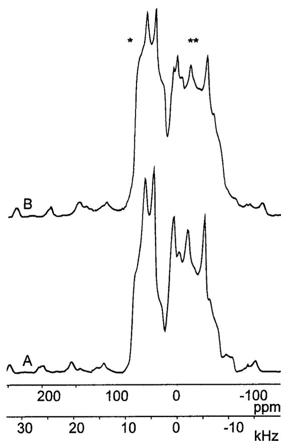
FIGURE 5. Comparison between the experimental (B) and simulated (A)  $^{27}\text{Al}$  CT MAS line shapes of the sample SIL (sillimanite). The line shape of this natural sillimanite can only be explained taking into account the kyanite spectrum besides the  $\text{AlO}_6$  (\*\*) and  $\text{AlO}_4$  (\*) signals of sillimanite.
