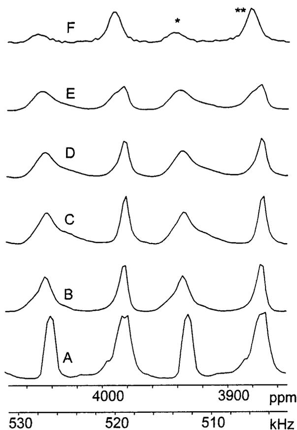
FIGURE 4. Plot of a few ST MAS spinning sidebands of SIL (sillimanite) (A) and the mullite samples CM1 (B), FM (C), CM2 (D), CM3 (E), and the sample GAM ( $\gamma$ - $\text{Al}_2\text{O}_3$ ) (F). Single star =  $\text{AlO}_4$  signal. Double star =  $\text{AlO}_6$  signal.
