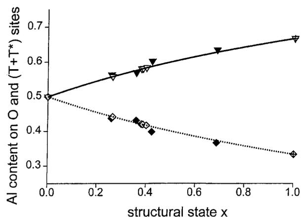
**FIGURE 8.** Octahedrally and tetrahedrally coordinated Al atoms normalized to the total Al content of the unit cell ( $\Sigma\text{Al}$ ) of mullite. Solid and dotted curves = structure model of Sadanaga. Filled diamonds =  $\text{AlO}_6/\Sigma\text{Al}$ ; filled triangles =  $\Sigma^{[4]}\text{Al}/\Sigma\text{Al}$ ; both are NMR results. Open diamonds = XRD; open triangles = neutron diffraction, both are average structure refinements.
