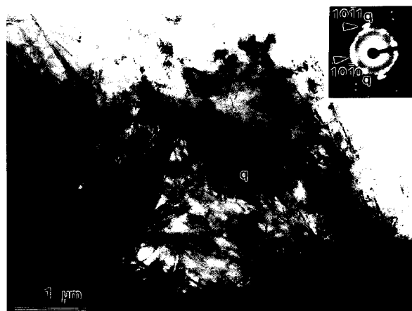
FIGURE 4. Bright-field TEM micrograph showing epitaxially grown quartz crystals (labeled q) on substrate of microfibrillar opal. Newly formed quartz grains display highly strained diffraction contrast. SAED pattern in inset reveals preferred orientation of quartz crystals presumably inherited from topotaxially transformed microfibrillar opal.
