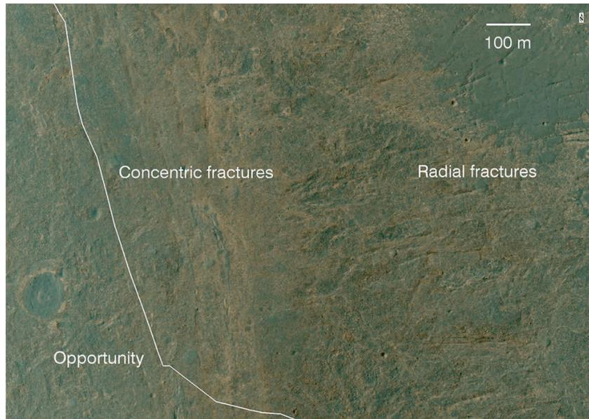
**FIGURE 3.** Portion of the HiRISE-based image segment covering Botany Bay, highlighting the locations of concentric fractures that are interpreted to have propagated up through the Burns formation outcrops just above a buried portion of Endeavour's rim between the Cape York and Murray Ridge rim segments. Radial fractures are evident extending to the east and northeast into Endeavour. HiRISE image ESP\_036753\_1775\_MRGB.
