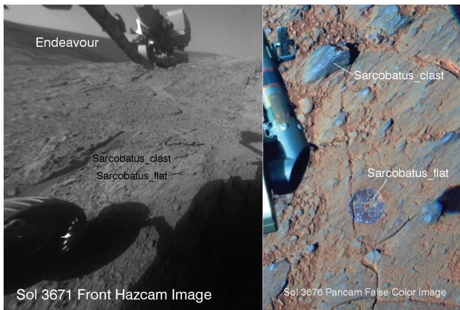
◀ **FIGURE 11.** Portion of a Front Hazcam image is shown on the left for the Sarcobatus in situ targets for a rock clast (two overlapping measurements) and the brushed matrix target (Sarcobatus\_flat). Pancam false color image of the targets is shown on the right. For reference the brushed spot is ~3.8 cm wide. Hazcam product ID 1F454088547FFLCDBAP1148R0M1. Pancam product IDs 1P454529822RADCDBAP2589L2C1, 1P454529907RADCDBAP2589L5C1, and 1P454529979RADCDBAP-2589L7C1.
