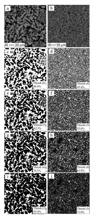
Supplementary Figure 1. Threshold testing for two different scales of AlK $\alpha$  X ray maps indicate that the difference small changes in image threshold can have an influence on calculated crystallinities (left column = 100  $\mu$ m²; right column = 500  $\mu$ m²). Threshold value and calculated proportion of crystals (black) are indicated for each image. Original gray scale images are shown in panels a and b.
