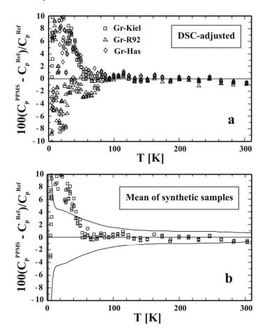
**FIGURE 9.** (Supplementary information) Percent difference plot between DSC-adjusted low-temperature heat capacity values ( $C_p^{PPMS}$ ) for synthetic grossular and published values ( $C_p^{Ref}$ ) obtained from adiabatic calorimetry (Haselton and Westrum 1980). (**a**) The three synthetic grossular samples Gr-Has, Gr-R92 and Gr-Kiel, (**b**) Their mean  $C_p$  values (the solid line is a ±1 $\sigma$  uncertainty envelope).
