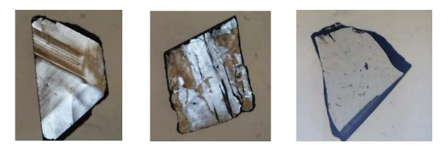
**FIGURE 1.** (Supplementary information) Photos, made under crossed polars, showing the optical properties of the three natural garnets. a.) Gr-44091, b.) Gr-82-112 and c.) Gr-L/K. The platelets range in size from about 2 to 3 mm in cross section.
