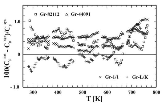
**FIGURE 15.** (Supplementary information) Percent difference plot between the high-temperature heat capacity values of natural grossular ( $C_p^{nat}$ ) and synthetic grossular ( $C_p^{syn}$ ) from data in this study. Natural garnets are Gr-82112 (squares), Gr-44091 (triangles), Gr-1/1 (X symbols) and Gr-L/K (crosses) (see Tab. 4).  $C_p^{syn}$  has been calculated using Eq. (4).
