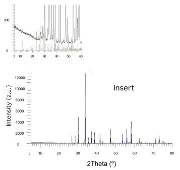
**FIGURE 3.** (Supplementary information) X-ray powder diffractogram for the sample Gr-Has (The other synthetic samples show similar patterns). Most of the very weak non-grossular reflections can be assigned to wollastonite or a wollastonite-like phase as shown, for example, by the arrows. The inset shows a portion of the diagram between 5 and 60° 2 $\Theta$   $\theta$ . Wollastonite peaks are marked by the vertical lines.
