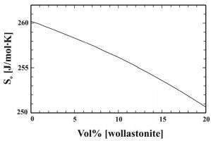
**FIGURE 17.** (Supplementary information) Plot showing the S<sup>o</sup> value for grossular as a function of the volume % wollastonite impurity (see text for further details).
