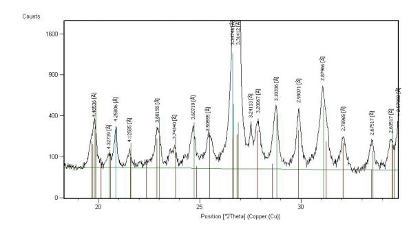
**Figure 5.** XRPD diagram of a phengite concentrate (99% purity) of the sample CHIVE-5 (operating conditions: 40 kV and 30 mA;  $54\text{--}64 2\theta$  range; step scan mode, with step width increments of  $0.02^{\circ} 2\theta$ , and step counting time of 2 s).
