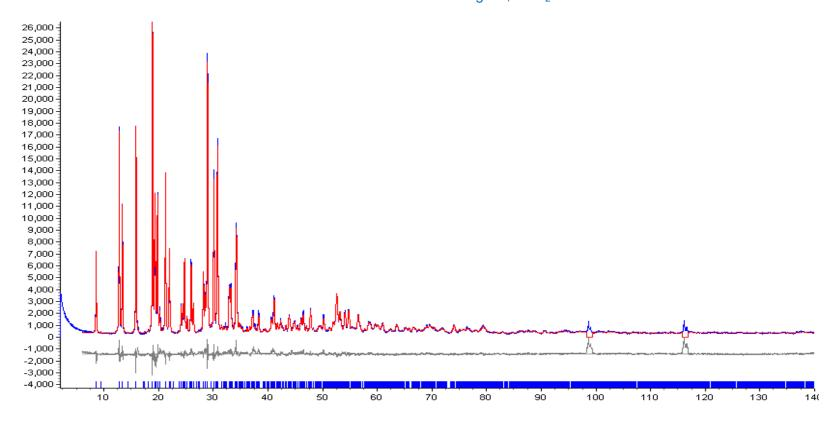
Red, Blue, and gray curves are calculated, measured, and difference curves, respectively. Blue bars are calculated peak positions.
