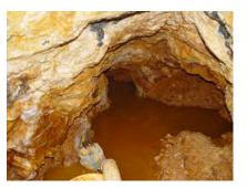
This chamber too ended in a curtain of quartz. Once more we drilled and shot a few holes. Another small cavity opened up with a suspicious opening at the back. After emptying this new chamber, and increasingly Houdini like feat to dig it out, we thrust a 1 meter nylon par into the softball sized aperture at the far back. It entered easily. For the third time we shot the roof of the cavity. This time though rather than revealing
