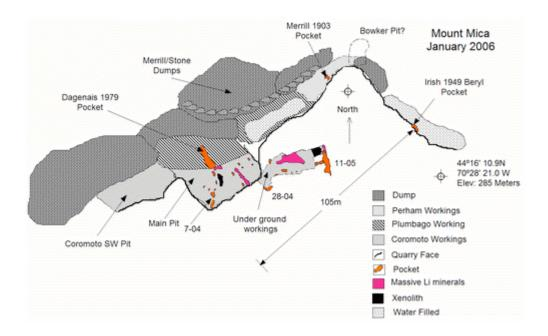
As described in a prior update to the PIG site, late in 2004 we started to mine underground beginning in the SE corner of the main pit. An adit was started in essentially a southerly direction between the eastern pit face and a large bloom of lepidolite and pollucite in the southern quarry face. This area of intensification of the mineralization in the pegmatite had occurred just up strike
