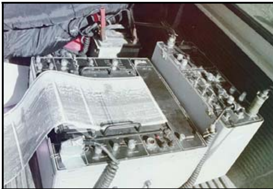
Figure 7: GSSI Model 4400R GPR unit and Model SR-8100H Graphic Recorder. The GPR unit is powered by a 12 volt D/C gel-cell battery. The Graphic Recorder is powered by 110 volts A/C.
