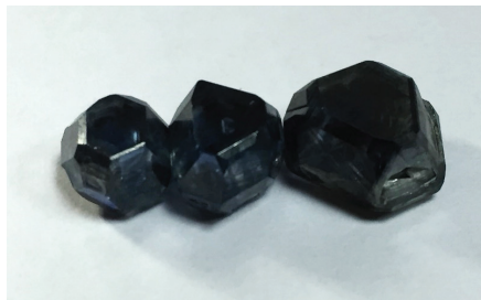
Figure 13. Deep blue to black Type IIb HPHT diamonds grown on {111}-oriented diamond seeds. Sizes range from approximately 6 to 15 ct. The upper face has a {111} orientation, reflecting that of the seed. The sizes and orientations of the other faces depend on the pressure and temperature conditions in the growth cell. [HPHT diamonds synthesized and photographed by ANK.]
