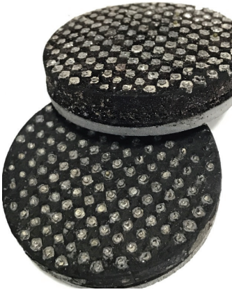
Figure 11. Typical example of HPHT diamonds resulting from multiple seed and multiple layer growth methods. The view is from the seed side (the bottom of the reaction volume illustrated in Fig. 2b), where the growth medium has been partially dissolved by acid cleaning. Average crystal size is ~4 mm each. [Diamonds grown and photographed by ANK.]
