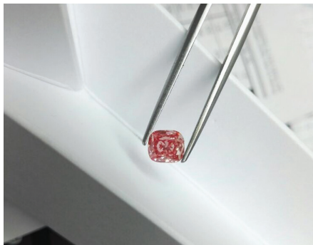
Figure 15. 2.55 ct HPHT-grown gem diamond with a saturated pink color due to high concentrations of nitrogen-vacancy centers. These color centers were obtained by a multi-step process: the original Type IIa + Ib HPHT diamond, containing a low concentration of substitutional nitrogen, was first electron irradiated and finally annealed at a moderate temperature. [HPHT diamond produced and photographed by ANK.]
