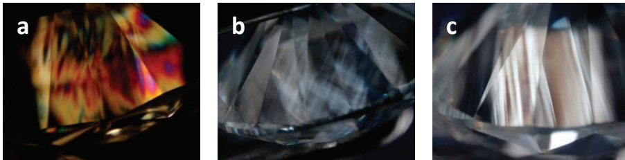
Figure 38. Strain birefringence patterns for faceted CVD diamonds can be (a) patchy, (b) tatami-like or (c) banded, making them difficult to separate from natural diamonds (e.g., Fig. 34a,b). These samples are characterized as follows: (a) 0.28 ct, H color, VS 2 clarity (field of view 3.10 mm); (b) 0.47 ct, G color, VVS 2 clarity (field of view 4.33 mm); and (c) 0.70 ct, I color, VVS 2 clarity (field of view 5.11 mm). [Photomicrographs by Wuyi Wang for GIA.]
