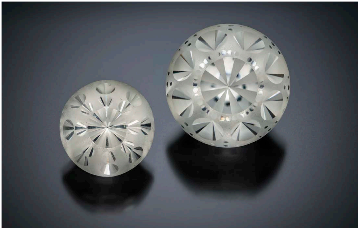
Figure 2: Compared to calcite’s birefringence of 0.124, that of quartz is relatively low at 0.009. Nevertheless, doubling will still be visible if the specimen is large enough and is viewed at the correct angle to maximize the effect. Here the larger 71.49 carat stone’s table facet is inclined approximately 45 degrees to the optic axis, there is maximum doubling, but mid-range partial birefringence. The effect is noticeable on the pavilion facets at the back of the stone as seen through its table; maximum depth is 20.15 mm at the culet (center point). The table facet of the smaller 29.39 carat quartz is cut in a plane parallel to its optic axis. Looking in a plane perpendicular to the table surface, there is maximum birefringence, but zero doubling of the pavilion facets. Both stones were cut by Art Grant and were part of the collection of Harold Dibble. The smaller stone was cut from a left-handed crystal and the larger stone is from a right-handed crystal (for more on handedness, see Skalwold and Bassett 2015); 19.20 x 15.55 and 25.50 x 20.15 respectively. Photo: Jeff Scovil.
