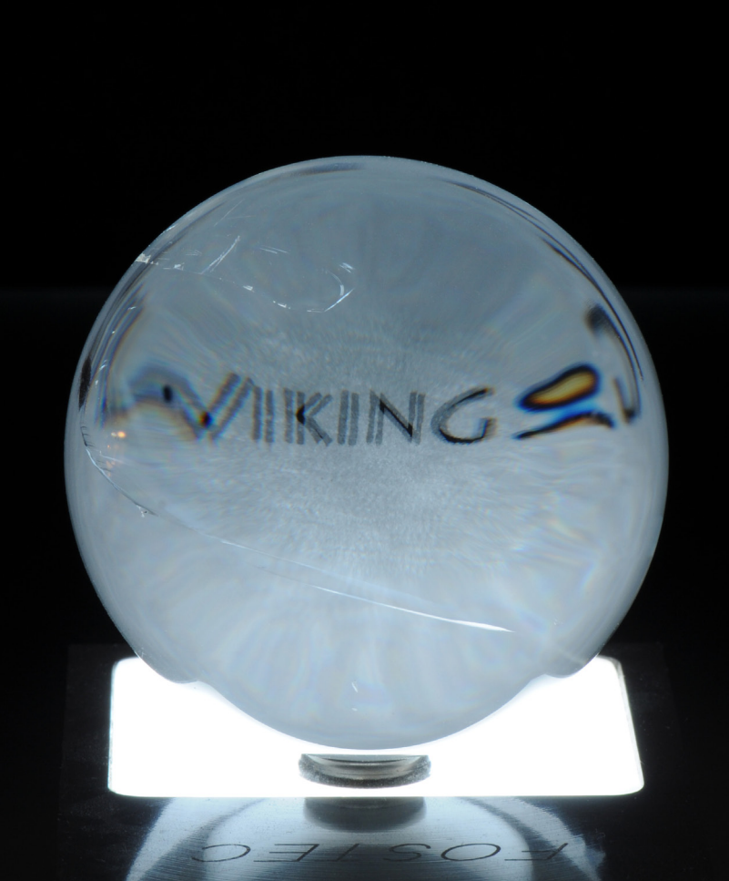
Figure 3: Maximum doubling is seen at approximately a 45 degree angle with the optic axis in this 60 mm quartz sphere.
