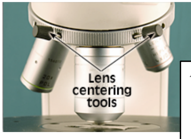
Figure 6: Placement of centering screws (Fig. 17.5, Dyar and Gunter 2008)
