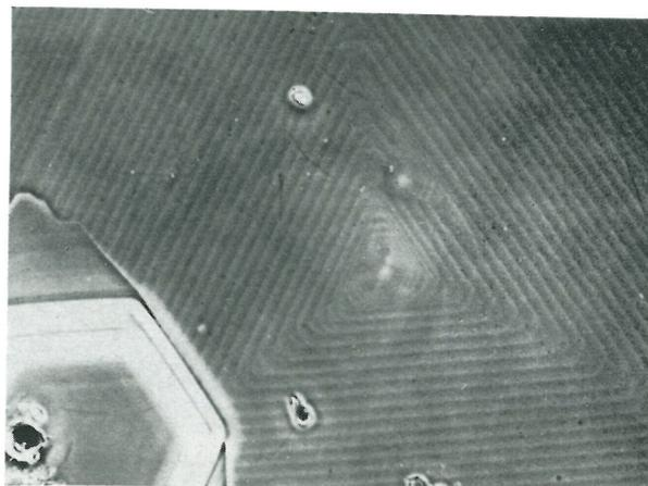
FIG. 2. Triangular spiral, positive phase contrast,  $\times 1000$ .
