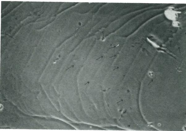
FIG. 9. Positive phase contrast photomicrograph showing triangular tongues projecting along the fronts of triangular thin growth layers. Arrows show the tongues,  $\times 250$ .
