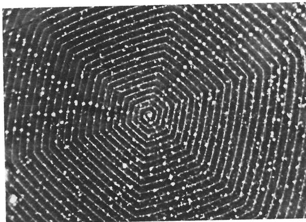
FIG. 3. Hexagonal spiral belonging to 6H polytype, positive phase contrast,  $\times 1000$ .
