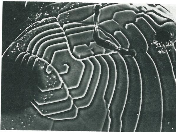
FIG. 1. Hexagonal spiral, positive phase contrast,  $\times 250$ .
