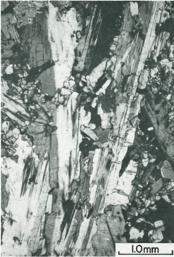
FIG. 7. Branching bytownite crystals from Willow Lake layer. Note discontinuous, bladed albite twins.
