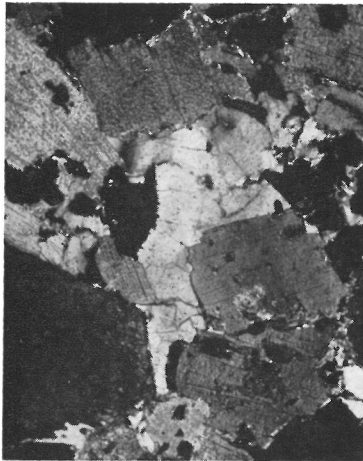
FIG. 8. Interstitial quartz (center) molded on biotite and on allanite (lower left). (39685), 18 \times , crossed polars.
