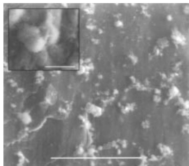
**FIGURE 5.** Scanning electron micrograph of many microorganisms on an anorthoclase surface left in situ for ~14 months. Inset is close-up of microorganism resembling *diplococcus* with weathering visible around the attached body. Bar scale = 5  $\mu\text{m}$ .
