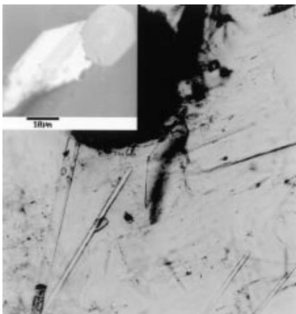
**FIGURE 2.** Transmitted light micrograph of anorthoclase showing abundant needles of apatite and oxide (magnification = 200 $\times$ ). Inset shows BSE image of apatite inclusion intergrown with Fe-Ti oxide.
