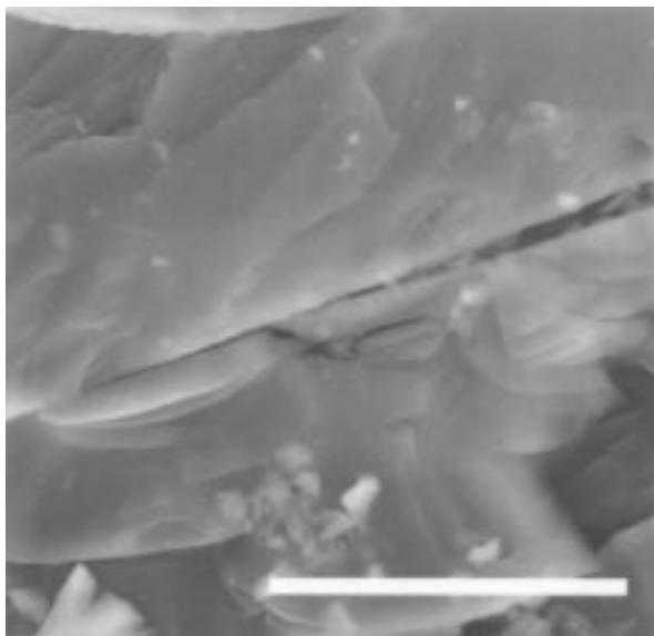
**FIGURE 3.** Scanning electron micrograph of a specimen of plagioclase after ~1 year in the contaminated region of the aquifer. No visible etching is observed on the surface, and no evidence of biological material or adhering microorganism. Bar scale = 15  $\mu\text{m}$ .
