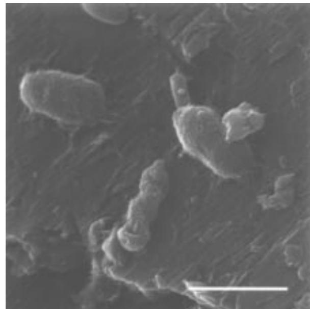
**FIGURE 4.** Scanning electron micrograph of anorthoclase left in situ for 4 months. Two types of microorganisms are present with a non-viable (dead) organism near the center of the image. Light etching of the mineral surface is visible. Bar scale = 2  $\mu\text{m}$ .
