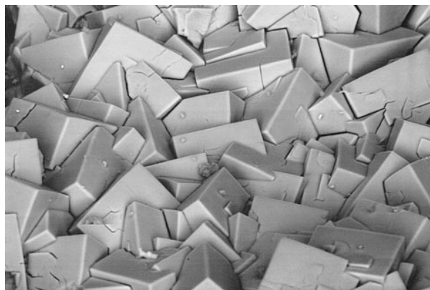
FIGURE 1. Scanning electron microscope micrographs showing the cubic habit of phosphovanadylite.
