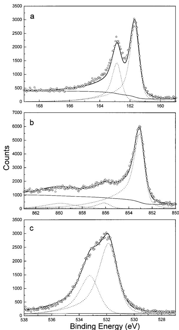
**FIGURE 3.** XPS S 2p (a), Ni 2p<sub>3/2</sub> (b), and O 1s (c) narrow region scans of millerite reacted with de-ionized water for 24 h. See Figure 2 for symbols.
