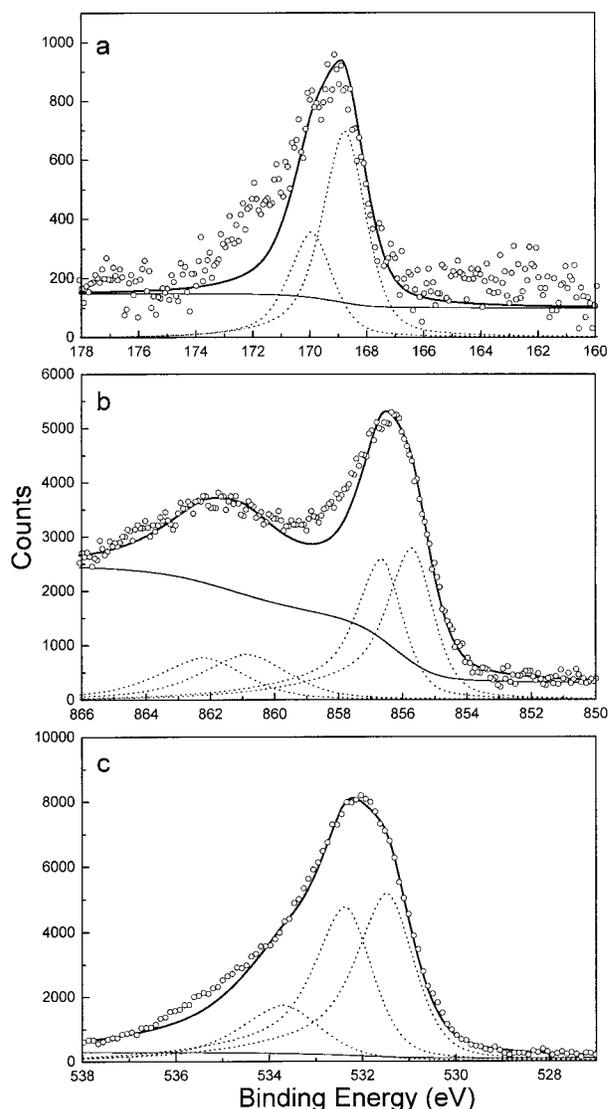
FIGURE 5. XPS S 2p (a), Ni 2p<sub>3/2</sub> (b), and O 1s (c) narrow region scans of millerite exposed to air on a lab bench for 1 year. See Figure 2 for symbols.
