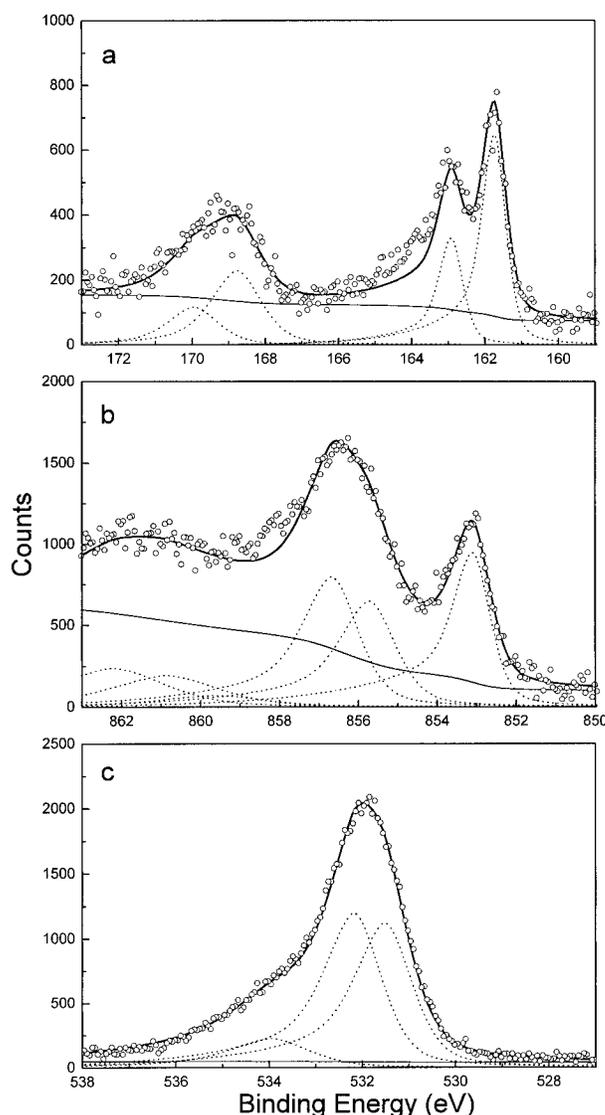
FIGURE 4. XPS S 2p (a), Ni 2p<sub>3/2</sub> (b), and O 1s (c) narrow region scans of millerite exposed to air on a lab bench for 24 h. See Figure 2 for symbols.
