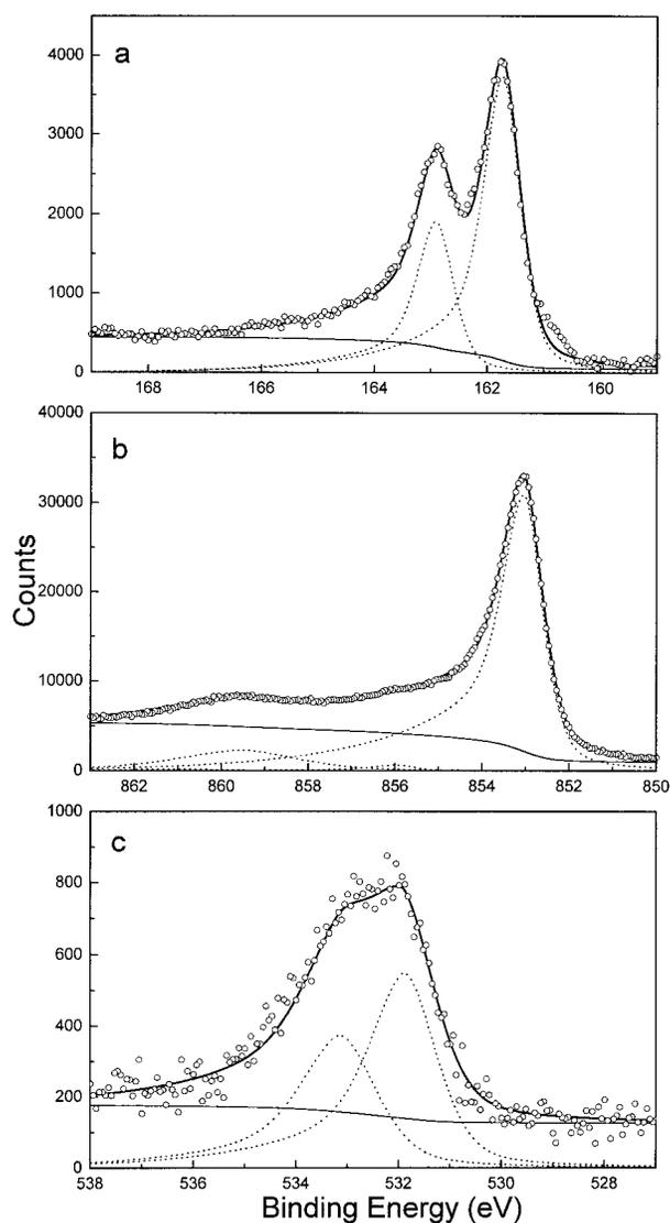
**FIGURE 2.** XPS S 2p (a), Ni 2p<sub>3/2</sub> (b), and O 1s (c) narrow region scans of millerite cleaved under vacuum in the analytical chamber of the XPS instrument. The open circles represent raw data. The thick solid line is the fit to the experimental data. The thin solid line is the fitted Shirley background and the dashed lines represent photoemission peaks from the near-surface of millerite.
