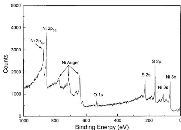
**FIGURE 1.** XPS broad scan of millerite cleaved under vacuum in the analytical chamber of the XPS instrument. The broad scan was collected immediately after cleavage. All major peaks are labeled. There is no detectable adventitious carbon contamination and oxygen is present in very small amounts. All other signals are derived from millerite.
