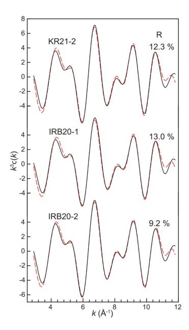
Figure SI4. Partial EXAFS spectra Fourier-filtered over the 0.8-3.3 Å R +  $\Delta R$  interval (black) with the optimum single-scattering simulations (red). R is the sum of the residuals, normalized to the sum of the data values.
