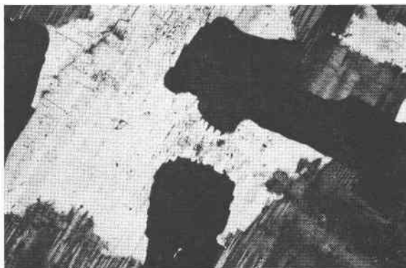
FIG. 11. Serrated borders between graphic quartz rods (black) and perthitic albite (light gray, faintly twinned). Microcline host is dark gray and twinned. Albite and microcline are crystallographically continuous. Crossed polars, 30X.
