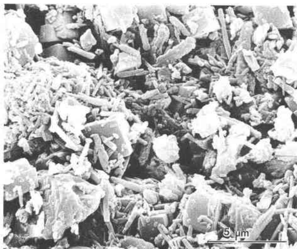
Fig. 1. SEM image of an intertidal carbonate assemblage from the Abu Dhabi sabkha (AD 31). Shown are aragonite needles and dolomite and magnesian calcite rhombs.
