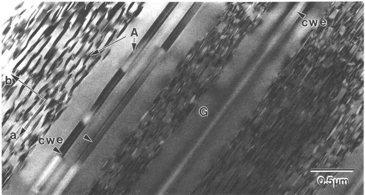
Fig. 12. Bright-field TEM image showing evidence for continual exsolution during cooling. The large straight lamellae formed first, nucleating on (010) CWEs, which run their entire length. As cooling progressed, the regions between the large lamellae became supersaturated with anthophyllite component. The region to the upper left of the image contains coarser lamellae than the areas between the large lamellae, and nucleation probably began in this area slightly before the nucleation of the smallest lamellae. The electron beam is near [001]. Microstructure from sample 89-27.
