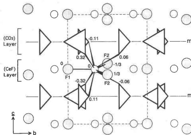
Fig. 1. Atomic arrangement of bastnäsite projected on (100). Triangles represent (CO<sub>3</sub>) groups, and O atoms in bastnäsite lie at the apices of the triangles; F atoms are stippled, and Ce atoms are depicted as open circles. (CeF) and (CO<sub>3</sub>) layers are denoted, and *x* coordinates of atoms are given. Dashed line outlines unit cell.
