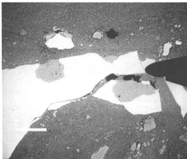
Fig. 1. Calcian alunite (gray) associated with pyrite (white) in matrix of sodian alunite (mottled gray). (BSE image, sample 109945.) Scale bar = 100 \mu\text{m} .
