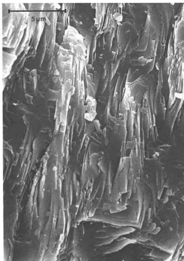
Fig. 1. SEM photomicrograph showing details from a cross section of a tvedalite spherulite. Note the platy habit of the mineral and its well-developed {010} cleavage. Elongation of the SEM photomicrograph is in the direction from rim to core.
