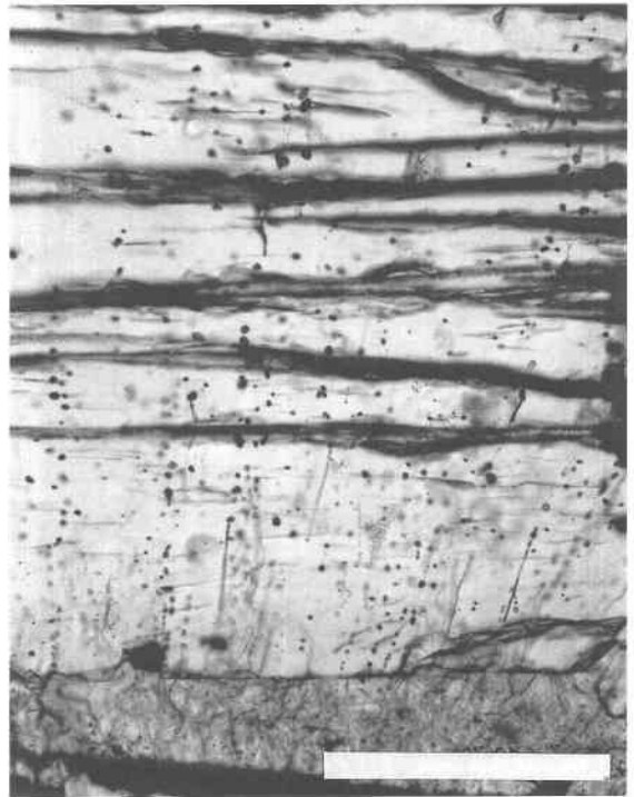
Fig. 1. Transmitted-light photomicrograph of the lower half of specimen VIII-2A, annealed at 2.0 GPa and 1200 °C in the presence of \text{CO}_2\text{-H}_2\text{O} for 14 d. Scale bar = 1 mm. Tubes (etch tunnels) and linear arrays of fluid inclusions emanate from the bottom of the olivine single crystal (just above the scale bar; the single crystal is in direct contact here with polycrystalline olivine) and extend in a radial fashion roughly parallel to [010]. Several of these linear arrays of fluid inclusions can be traced to tubes in the process of necking down. The dark horizontal lines are cracks produced during the quench.
