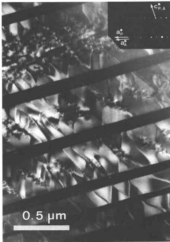
Fig. 1. Dark-field ( g = 102 ) electron micrograph and electron diffraction pattern of the Hakone pigeonite with coarse, heterogeneously spaced "001" augite lamellae.
