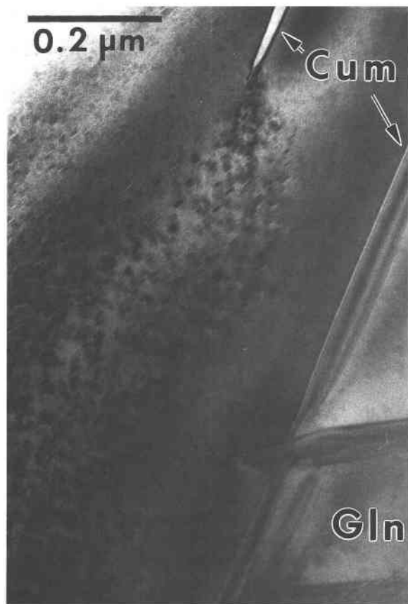
Fig. 4. TEM image of GP zones in the area between coarse cummingtonite lamellae. These tiny platelets probably nucleated homogeneously in an area that has become supersaturated with respect to Fe-Mg. Precipitate-free zones can be seen adjacent to the larger lamellae. A nonzone-axis orientation was used to enhance contrast.
