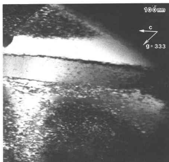
Fig. 4. Dark-field image ( g = 333 ) showing coexistence of both fine-scale domain structure and larger domains.
