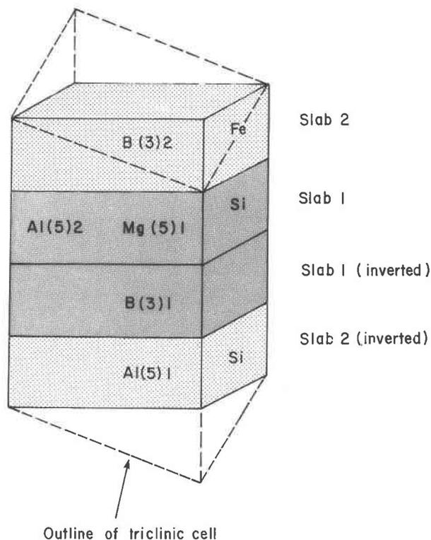
Fig. 4. Relationship of the triclinic unit cell (dashed outline) to the mullite-like slabs shown in Figure 3.
