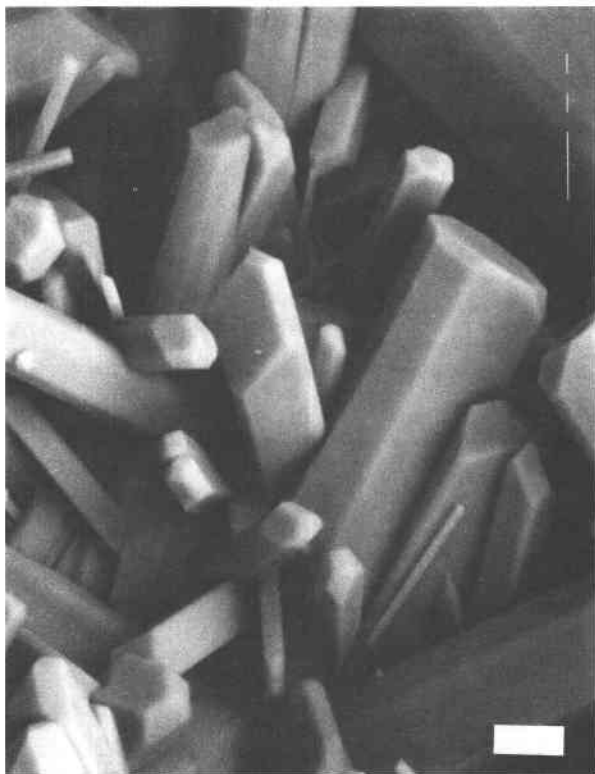
Fig. 1. Scanning electron microscope photomicrograph showing ashburtonite crystals elongated on [001]. Scale bar is 10 \mu\text{m} .
