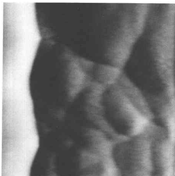
Fig. 3. Closeup along the edge of a small pit imaged in H_2O . This pit probably resulted from a fluid inclusion. In top view images such as this, darker tones represent increasing depth; maximum pit depth in image = 15 Å. Maximum relief along bottom of pit = 7 Å. Image dimensions = 210 × 210 nm.
