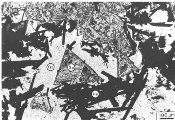
Fig. 2. Photomicrograph of the genthelvite + quartz + hematite (Ge-Qz-He) association. Note that genthelvite crystals show a perfect tetrahedral shape and that the euhedral hematite laths and xenomorphic quartz crystallized after genthelvite.
