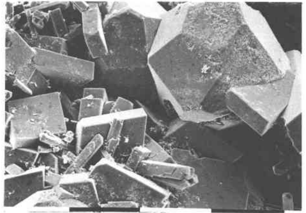
Fig. 4. Scanning-electron-microscope view of last-deposited calc-silicate phases showing wairakite (didodecahedral) intergrown with prehnite; crystal needles are of epidote. Scale bars are 0.1 mm long.
