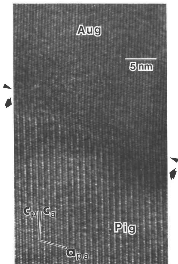
Fig. 4. A b -axis HRTEM image showing relative axial orientation and bending of fringes at the coherent interface of a “001” pigeonite-augite exsolution lamella. The lower set of arrows indicates the trace of the boundary, and the upper set indicates where most of the bending of fringes takes place.
