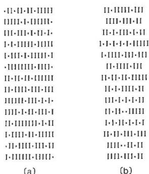
Fig. 9. Arrangements of interlayers (a) calculated on the basis of Markov theory and (b) random accumulations of fundamental particles for sample LPB.
