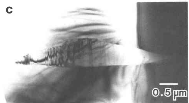
Fig. 6. Amphibole lamellae showing deviations from the usual (100) interface orientation with orthopyroxene. (a) An irregular interface. (b) An amphibole lamella exhibiting a pronounced change in width. (c) A lens-shaped amphibole lamella. Vertical features in the amphibole lamellae of a, b, and c are all chain-width errors in different contrast.
