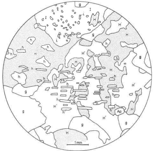
Fig. 3. View of microstructure in specimen 5, showing dolomite rods (i) enclosed by optically continuous calcite (I), dolomite plates (h) enclosed by optically continuous calcite (H) and optically discontinuous calcite (H'), and discrete grains of dolomite (g) some of which may be of exsolution origin. Ap = apatite.
