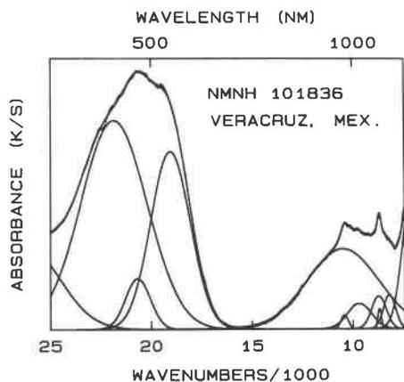
Fig. 1. Diffuse-reflectance spectra and model deconvolution of NMNH 101836. Bands at 10 400, 18 800, 20 600, and 22 400  $\text{cm}^{-1}$  result from electronic transitions of  $\text{Mn}^{3+}$ . The weak, sharp bands near 9000  $\text{cm}^{-1}$  are overtone and combination bands of interlayer  $\text{H}_2\text{O}$  and structural OH.
